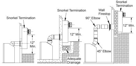
Figure 16 - Snorkel Termination Configurations for Below Ground Installation www.desatech.com
